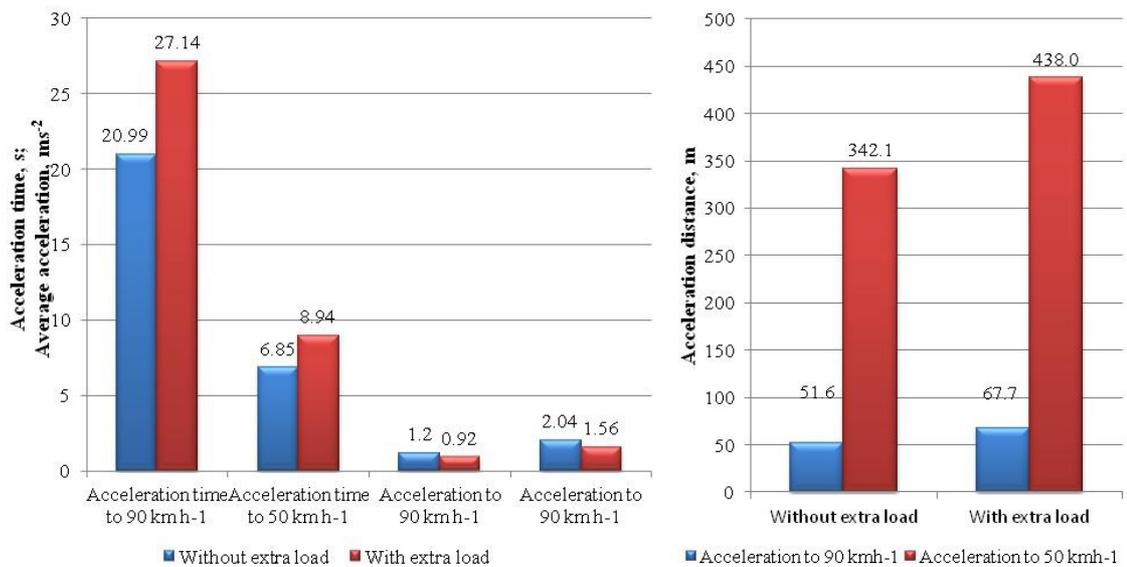
Fig. 6. Key characteristics for the acceleration of the electric automobile
